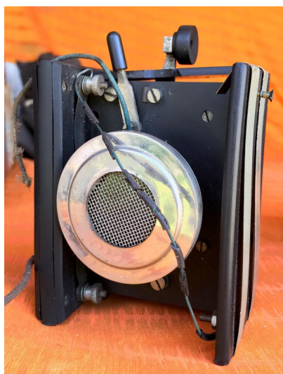
Photo 5 - Medhurst Field Telephone
